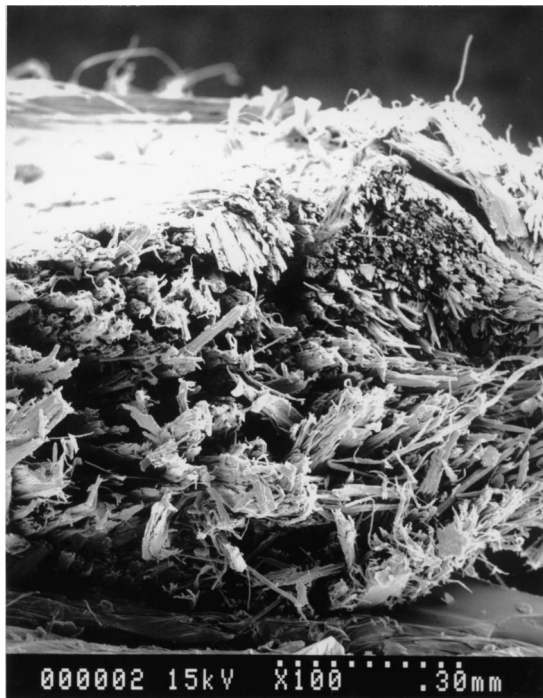
Fig. 4. SEM photograph of fractured surface of VB/MA-PP binary blend at the draw ratio of ca 1.
